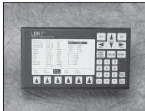
The optional LBK1 remote operation terminal provides control of the LogBook/300 system in the field when no PC is present
